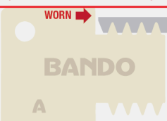
Fig 2: Worn Belts (Red Line is Reference Level)
