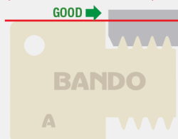
Fig 1: Good Belts (Red Line is Reference Level)
