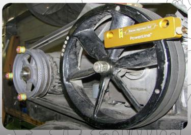
L80 Laser Alignment Tool Align belts and pulleys, as well as a variety of other power transmission components with confidence, speed and accuracy **BUI 4018**
